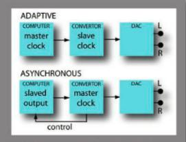
In Adaptive mode the convertor has a low jitter clock, phase-locked to the computer clock. In Asynchronous mode roles are changed: a stable, jitter free convertor clock takes charge, feeding the DAC a perfectly clocked data stream. The computer is controlled by the convertor.
