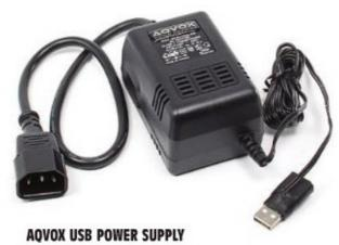
This USB power unit supplies 5V at 1A to a USB line by breaking the power connection from the computer and inserting itself with an in-line adaptor plug – a neat idea. Rafael used it with the Halide Bridge convertor and felt they worked well together.
